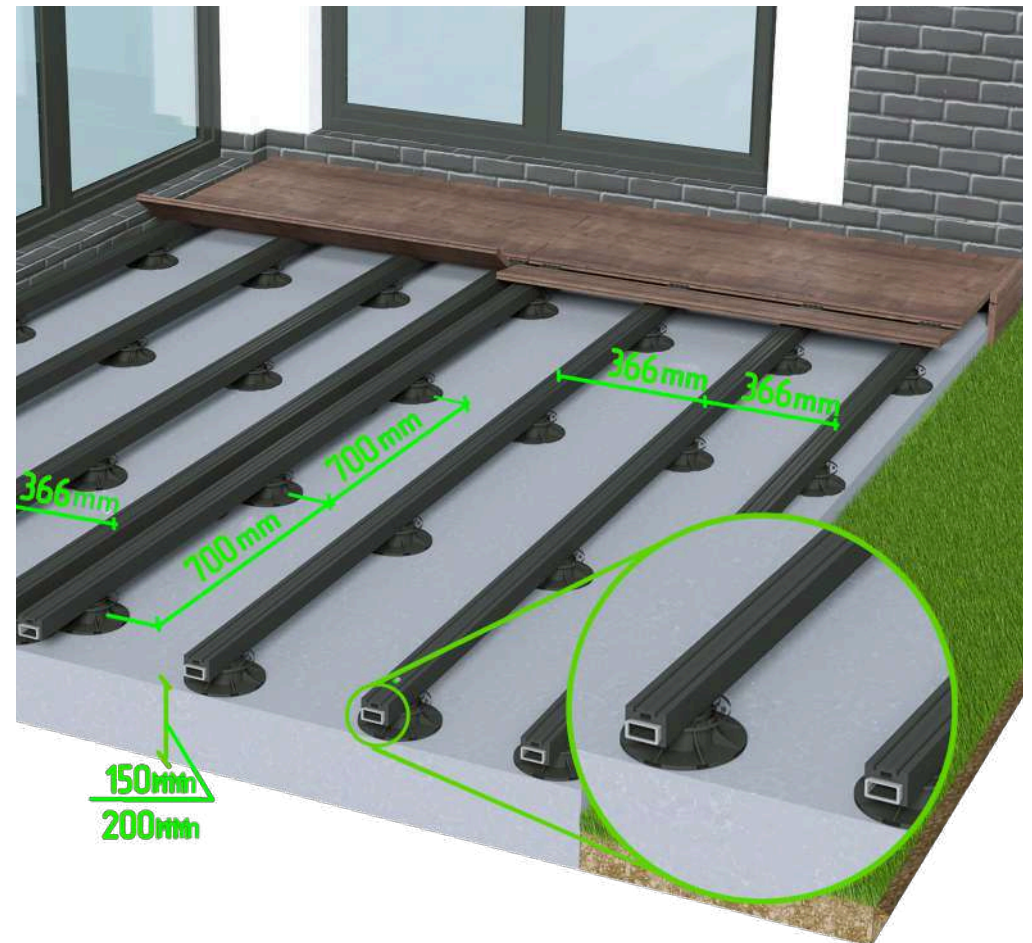
Installation of a reinforced log on plastic adjustable supports.
