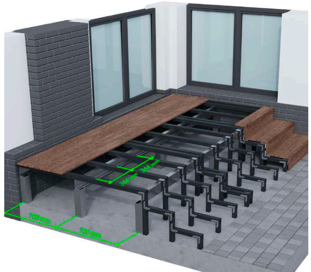
Installation of the board on a combined structure (metal frame and reinforced strengthened WPC log).
