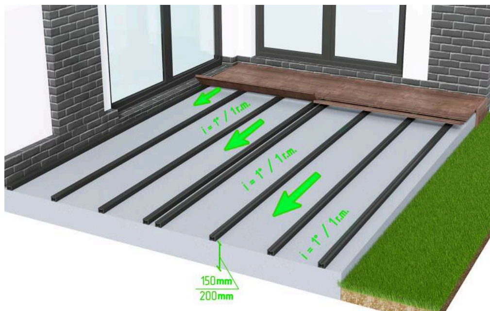
Installation of a standard log on a concrete base with a slope.
