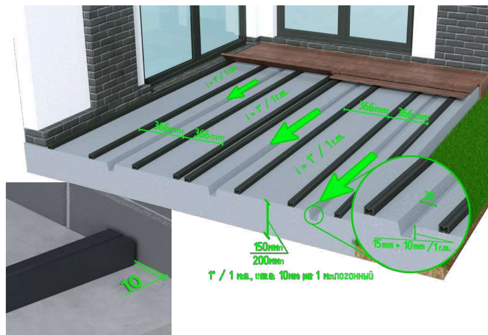
Installation of a standard log on a concrete base without a slope with a system of drainage channels.
